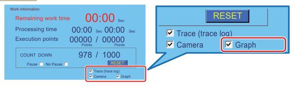
When the **[Graph]** is checked, the graph of the tip temperature of the SOLDER UNIT will be displayed on the software top screen. When the **[Graph]** is unchecked, no graph will be displayed but the Trace function continues recording the tip temperature.
