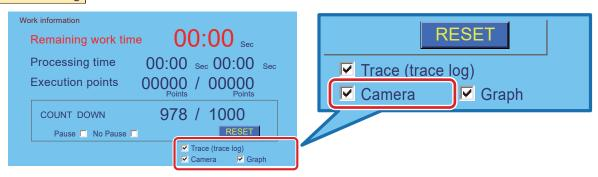
When the **[Camera]** is checked, the image of the selected camera will be displayed on the software top screen.
