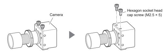
**2.** Fix the camera to the arm with the screw (M2.5  $\times$  5) in Step **1**.
