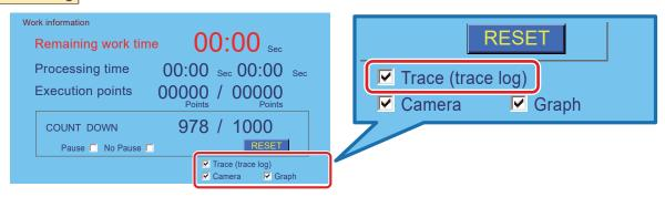
When the [Trace] is checked, the software will record soldering operation during program run.
