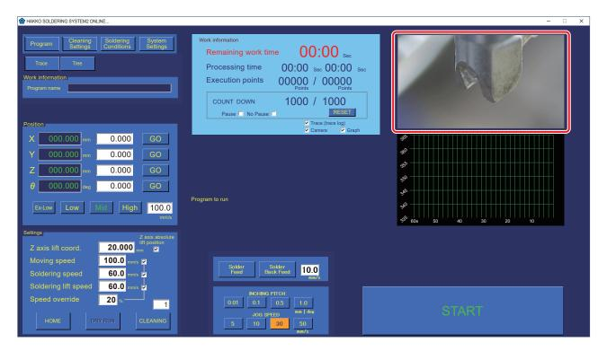
**3.** Adjust the arm/camera to the camera footage until the camera is in focus.
