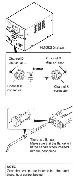
Both tips of the set must be inserted or the handpiece will not heat.
