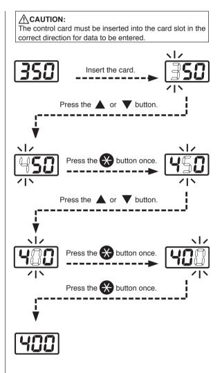
When the station is ON and the control card is in the station, the data entry procedure is:
