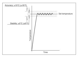
Figure 1. Temperature accuracy and stability.
