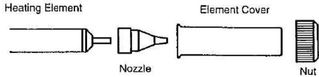
Remove the nut with the attached spanner.
