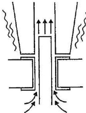
Absorb the solder by slowly moving the lead back and forth with the tip of the nozzle.
