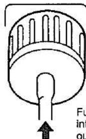
Fully insert the hose into the vacuum outlet cap.
