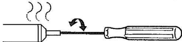
The cleaning pin passes cleanly and completely through the hole.
