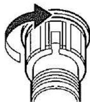
Secure the plug by turning it clockwise.
