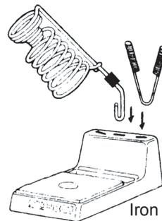
Iron Holder for Desoldering Gun
