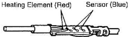
1. Turn the unit ON and set the temperature control knob to 480°C (896°F). Then wiggle and kink the iron cord at various locations along its length, including in the strain relief area.
