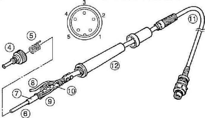
1. Turn the nut (1) counterclockwise and remove the tip enclosure (2), the tip (3).
