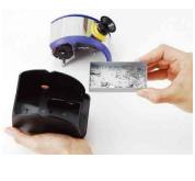
The safety design requires removal of the AC adapter to take off the cover.
