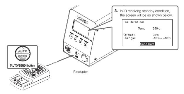
**5.** If the measured data is within the set range it will be judged as passed. If it is outside the set range, temperature measurement and sending will be performed repeatedly for the previously set number of retries.
