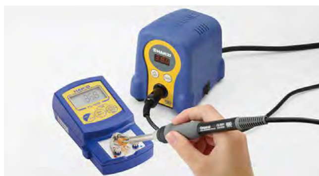
Measuring the tip temperature with a tip thermometer (FG-100B)
