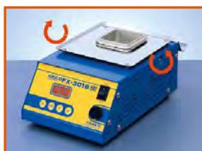
Loosen the screw on both sides.
