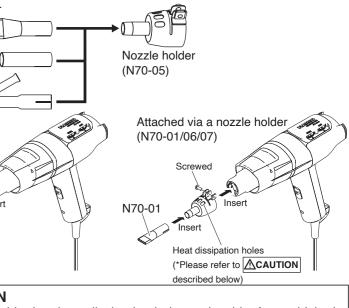
The nozzle holder has heat dissipation holes on its side, from which air will be exhausted that is at least as hot as the air from the nozzle. When attaching the nozzle holder to the unit, make sure that the holes are oriented to suit your work, being careful to prevent burn injuries.
