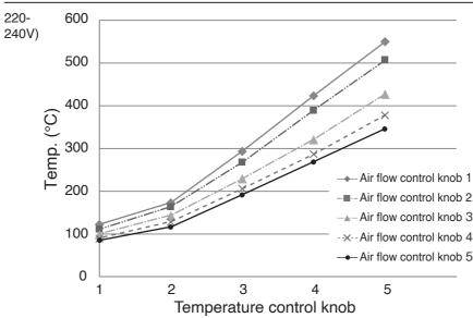
Measured at the point 10mm from the pipe. (without nozzle\*)
