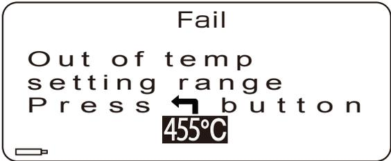
Failure display screen
