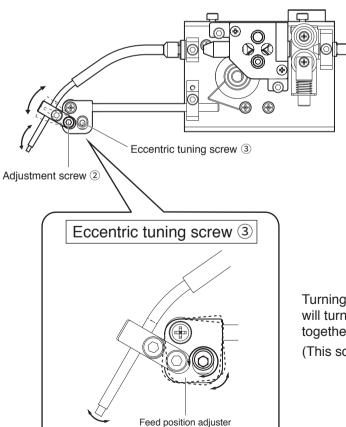
Turning the eccentric tuning screw ③ will turn the feed position adjuster together, allowing you to make tuning. (This screw cannot be removed.)
