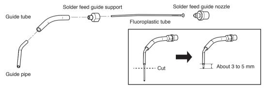
Turn the solder feed guide nozzle counterclockwise and remove the solder feed guide support. You can now install the fluoroplastic tube. Lastly, insert the guide pipe.
