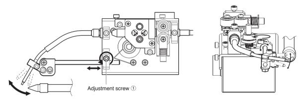
2. Loosening the adjustment screw ② will allow you to move the guide pipe as shown in the figure below. Move the guide pipe until solder comes into contact with the tip.
