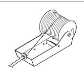
Ensure that solder is reeled out of the top of the bobbin.
