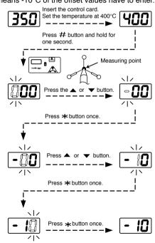
3. When change the offset values for MODE FM-2022 or MODEL FM-2023, refer to the above 1 and 2 procedure after measuring the tip temperature of either tip.
