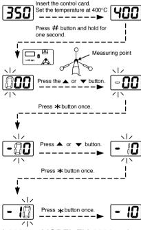
3. When change the offset values for MODE FM-2022 or MODEL FM-2023, refer to the above 1 and 2 procedure after measuring the tip temperature of either tip.
