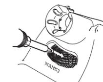
Material that is not removed easily with the cleaning sponge can likely be removed using the cleaning wire.
