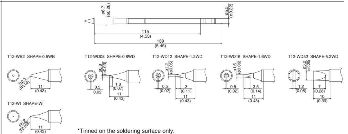
\*Tinned on the soldering surface only.
