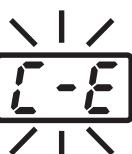
**C-E** will be displayed if the connector cord is not attached to the station OR the wrong soldering iron is connected.
