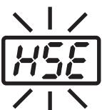
**HSE** will flash, and the buzzer will sound continuously, when the tip is inserted incorrectly, an incompatible tip is inserted, or a foreign object has found its way into the connector.
