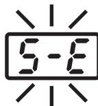
When there is the possibility that a failure has occurred in the sensor or heater (including the sensor circuit), **S-E** is displayed and the power is shut down.
