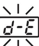
**d-E** appears on the display when turning the power on after connecting the MODEL FM-2022/2023 with a hot tip.
