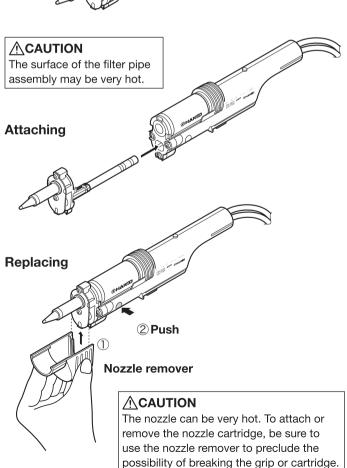
Press the nozzle unlock button (A) and remove the nozzle cartridge.
