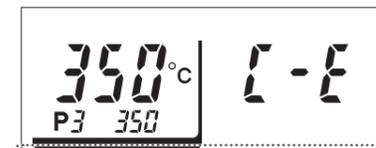
If no handpiece is connected to a channel, [C - E] is displayed and the buzzer will sound. If the channel button is pressed for 2 seconds, the display will change to [OFF] and the buzzer will stop. (See "Channel power ON/OFF" in "4-3. Operation")
