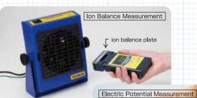
Ion balance can be measured in 1-V intervals.
