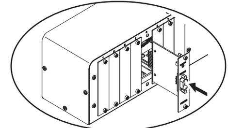
When attaching the interface card, be sure to insert the interface card while aligning the PWB position to the guide rail.
