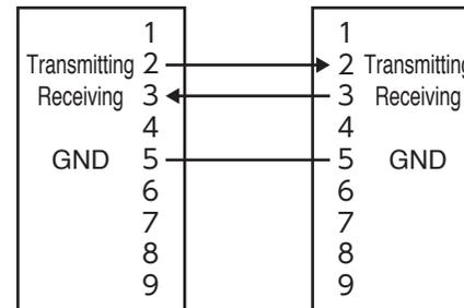
A cable of the Dsub9 pin straight connection is attached to the interface card (B5211) for FN-1010. Pins on the interface Card side except for numbers 2, 3 and 5 are unused, so, any straight-connection cables can be used.
