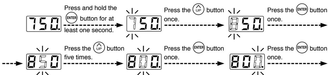
The desired temperature is saved to the system memory.
