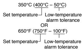
If the sensor temperature falls below the difference between the current temperature setting and the low-temperature alarm tolerance, **H-E** is displayed and the warning buzzer sounds. When the tip temperature rises to a value within the set tolerance, the buzzer will stop sounding.
