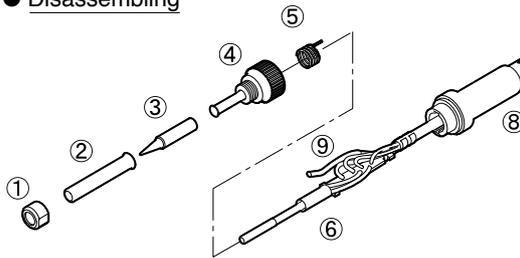
1. Turn the nut ① counterclockwise and remove the tip enclosure ② and the tip ③.
