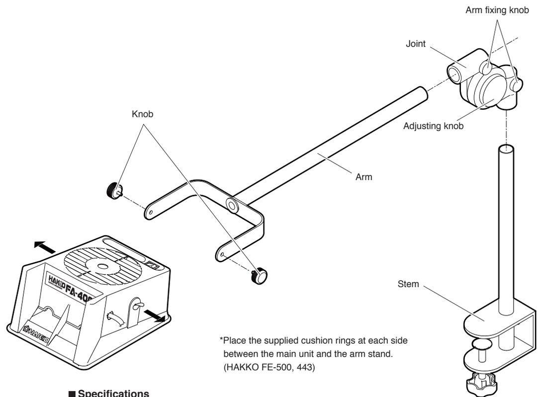
\*Place the supplied cushion rings at each side between the main unit and the arm stand. (HAKKO FE-500, 443)
